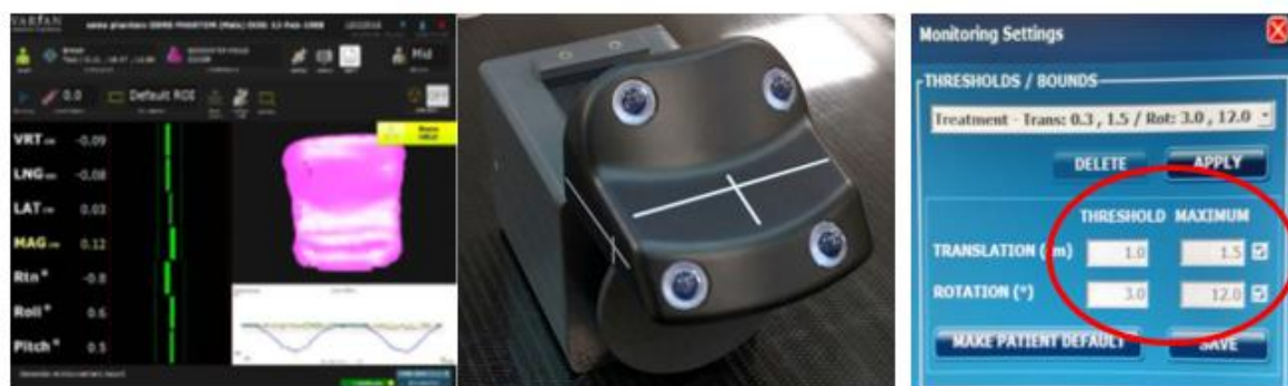
Figure 8: Dynamic Radiation gating delivery with threshold values to hold the beam.
