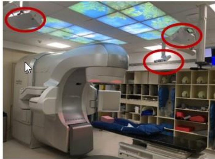
Figure 1: Display of Optical Surface Monitoring system installed on True BEAM STx
