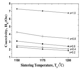
Fig. 8: Coercivity at different sintering temperatures.
