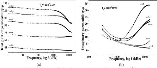
Fig. 3: (a) Real and (b) Imaginary part of permeability at  $T_s=1200^{\circ}C$ .
