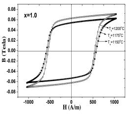
**Fig. 6:** B-H loop for all samples at  $T_s=1175^{\circ}C$ .
