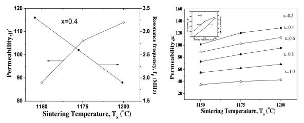
Fig. 4: Variation of permeability and resonance frequency with sintering temperature for x=0.4.
