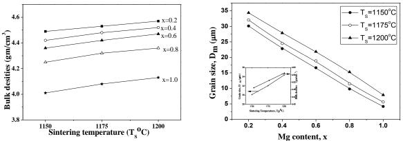
Fig. 1: Variation of bulk density with sintering temperature. Fig. 2: Change of grain size with Mg content.
