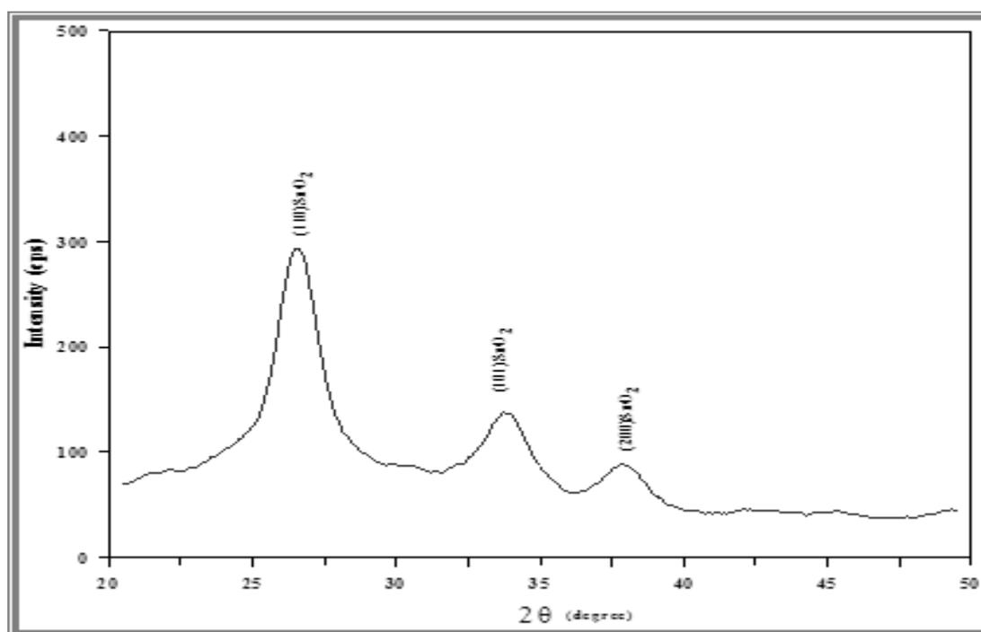
Fig. 3 XRD patterns for pure SnO<sub>2</sub>
