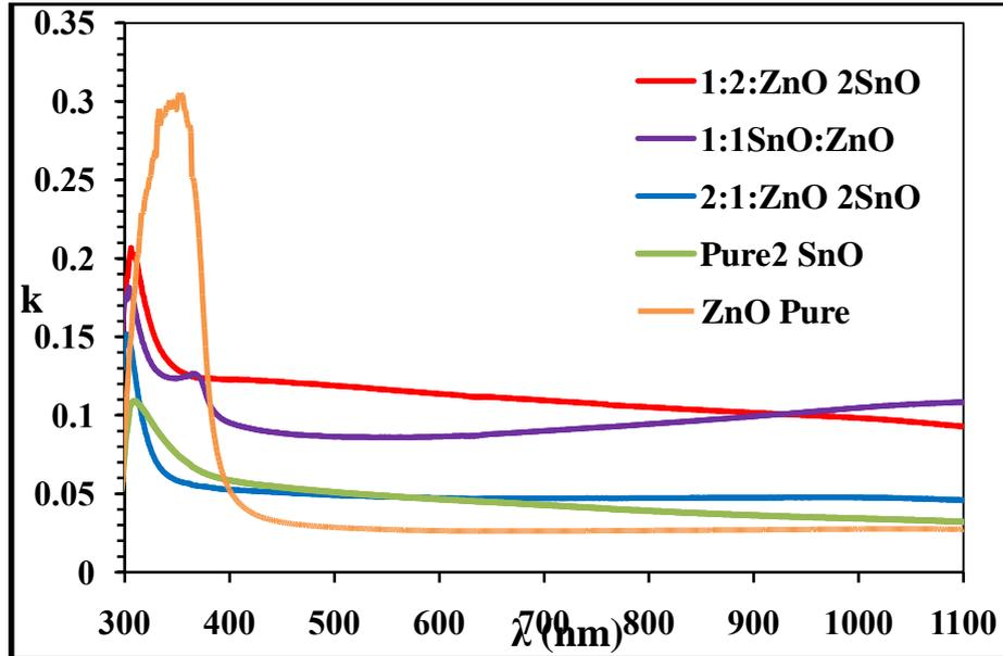
Fig.9. extinction coefficient spectra of ZnO/SnO<sub>2</sub> pure and their composition thin films deposited with different percentage.
