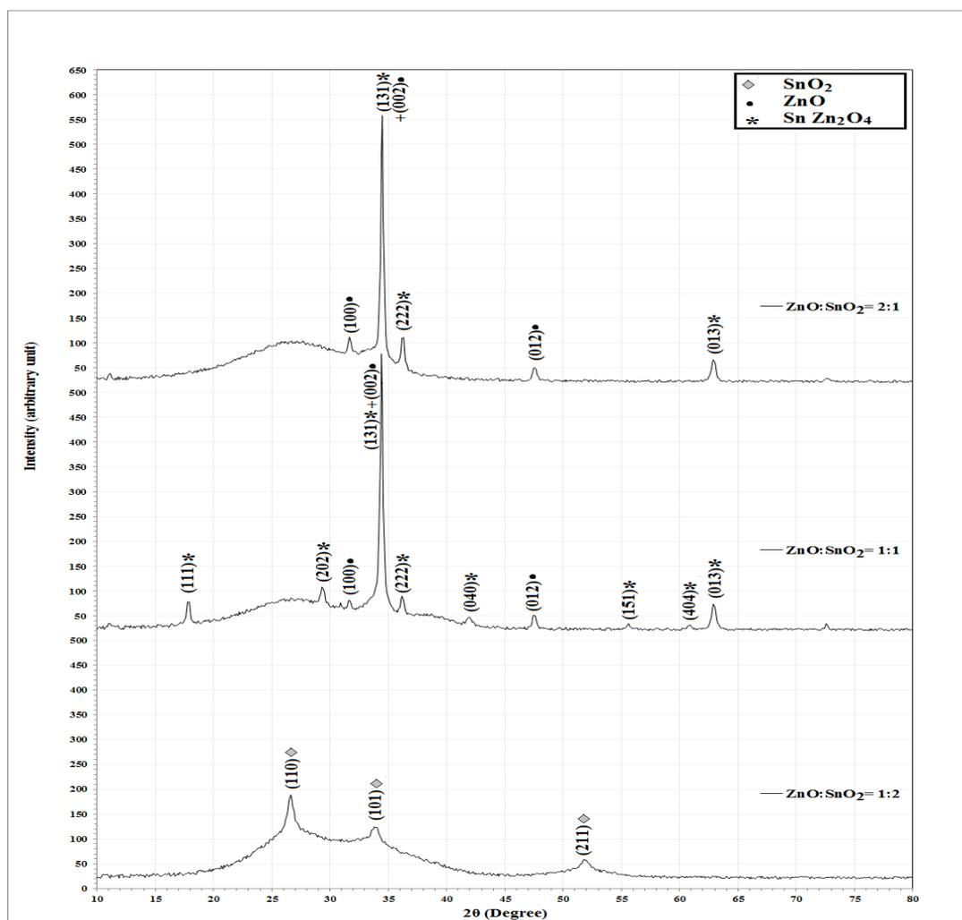
**Figure4** show the x-ray diffraction (XRD) patterns of the ZnO/SnO<sub>2</sub> composite films with different contents
