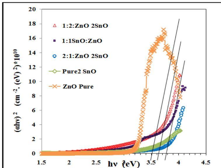
Fig.10: Optical band gap for ZnO/SnO<sub>2</sub> pure and their composition thin films deposited with different percentage.
