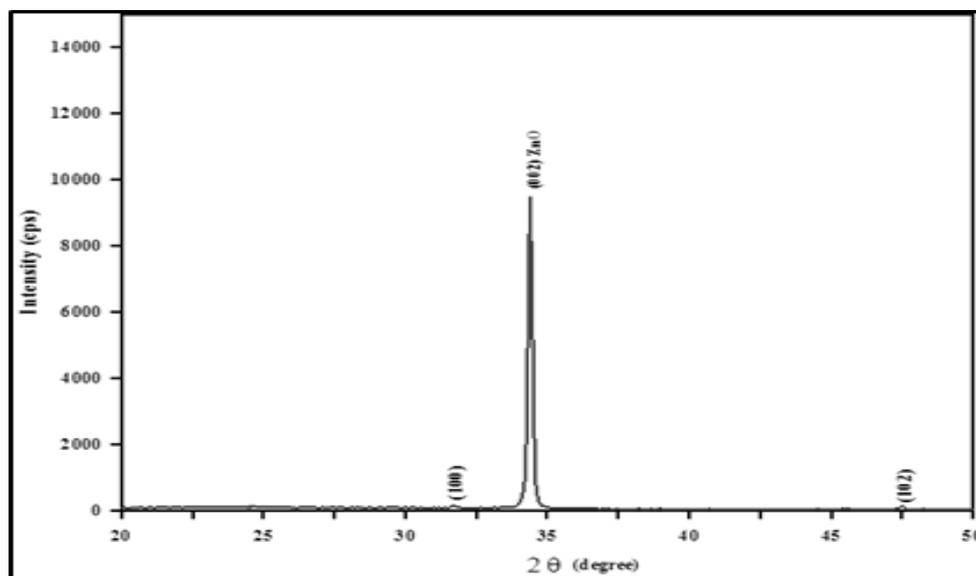
Fig. 2 XRD patterns for pure ZnO
