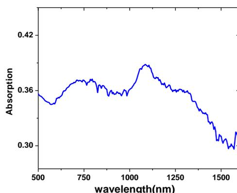
Fig.3. Measured experimental absorption spectra for the gold rods. Two absorption peaks can be observed indicating of the resonances at wavelengths of 781.2 nm with a peak of 37% and 1083.3nm with a peak of 39% respectively.
