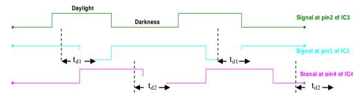
Fig. 7 Waveforms summarizing the flow signals of the system
