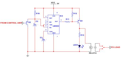
Fig. 5 Schematic diagram of the time delay unit and the switching unit
