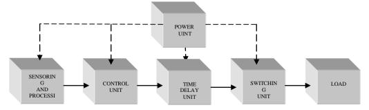
Fig.1the block diagram of the Automatic Household Electrical Lights Monitoring System.
