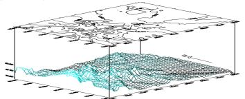
Fig.4: Physical shape of the earth surface of the study area with respect to mean sea level
