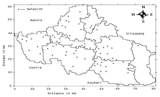
Fig.2: Distribution of static water level measuring points in the study area.
