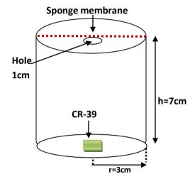
Fig.2: Schematic diagram of the optimum Radon.
