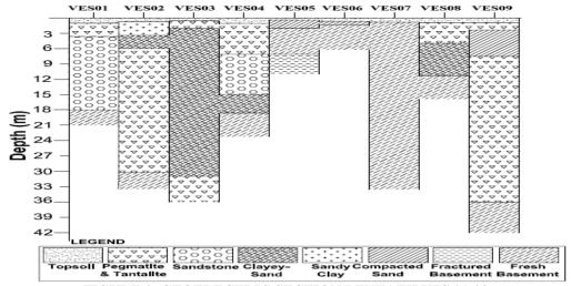
FIGURE 3: GEOELECTRIC SECTION BENEATH VES 01-09
