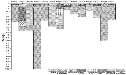
Figure 4: GEOELECTRIC SECTION BENEATH VES 10-23
