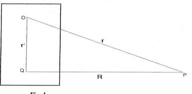
For far field radiation, the largest length of the source volume is small compared to its distances from the observation point in the radiation zone. If the origin O is taken within the source volume, then  $OP \approx OQ$  [Fig.1] and Poynting flux of energy S radiated from return stroke is written as
