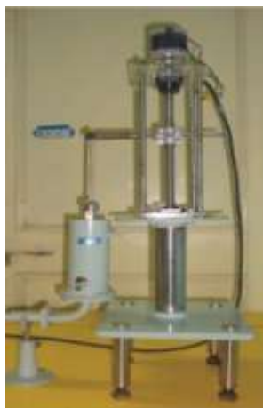
Fig.3: Experimental set-up with Labeling for Liquid cell of X-band Microwave bench
