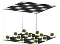
Fig. 1. A control volume with moisture concentration at two planes of observation at the base z=0 and top  $z=h_{cv}$
