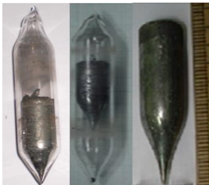
Entirely detached crystallization of Sb-based materials in the VDS process since 1994.
