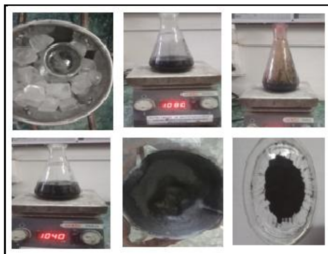
Fig. 3.4: Actual lab work for Graphene Oxide synthesis (Hummer's method)
