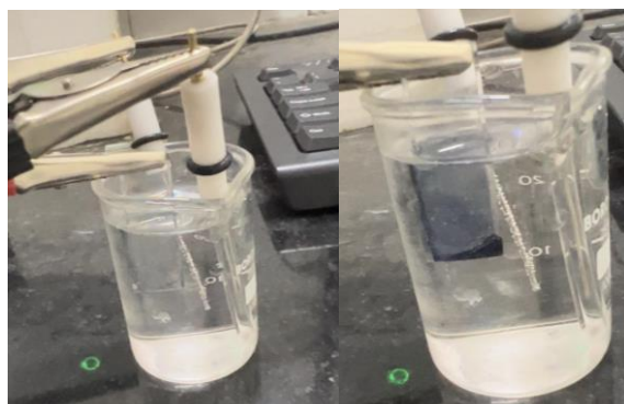
Fig 2.7 and 2.8 - change in state of \text{WO}_3 film from bleached to coloured during cyclic voltammetry
