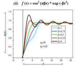
Fig.4 Intensity distribution curves for double filtering
