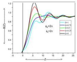
Fig.3 intensity distribution curves for single filtering
