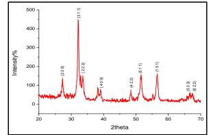
Fig. 2. Powder XRD pattern of the synthesized Cd2SnO4 nanoparticles
