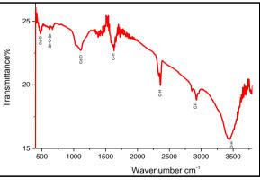
Fig. 6. FTIR spectrum of Cd<sub>2</sub>SnO<sub>4</sub> nanoparticles
