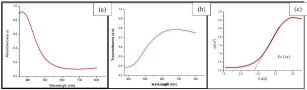
Fig.4(a)Opticalabsorbance(b)Transmittanceand (c)Tauc'splot of Cd<sub>2</sub>SnO<sub>4</sub> nanoparticles
