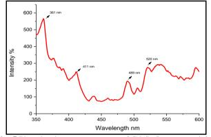
Fig. 5.Photoluminescence spectra of Cd<sub>2</sub>SnO<sub>4</sub> nanoparticles.
