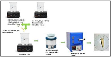
Fig.1.Graphicalillustration for the synthesisofCd<sub>2</sub>SnO<sub>4</sub>nanoparticles
