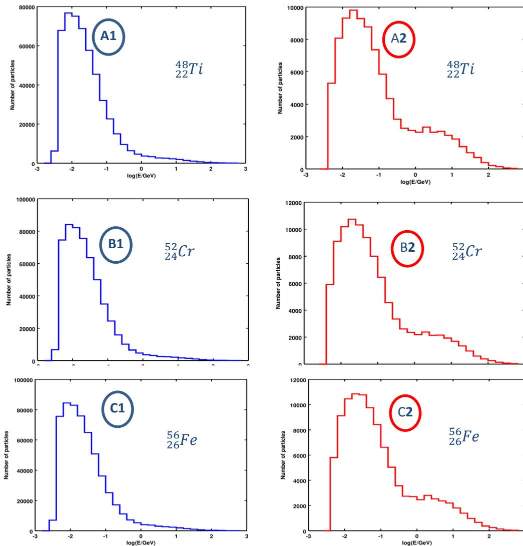
**Figure 3.** The spectra of  $\log(E/\text{GeV})$  of the EAS particles generated by CORSIKA 7.6400 for each of the heavy extraterrestrial nuclei selected for this study. The left column are the whole spectra, and the right column are the no-photon spectra.
