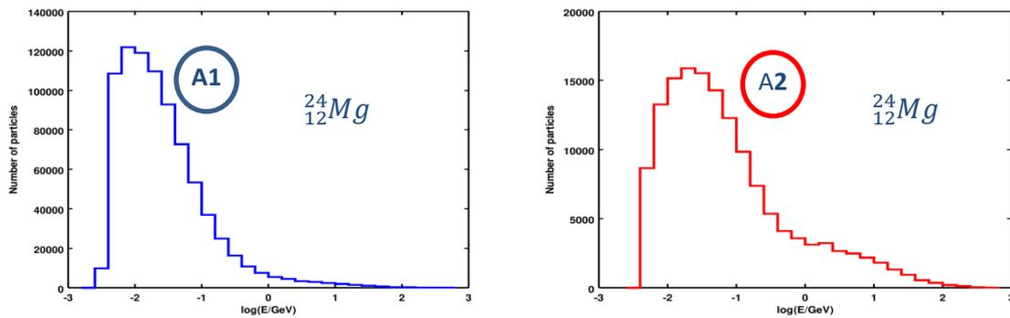
**Figure 2.** The spectra of  $\log(E/\text{GeV})$  of the EAS particles generated by CORSIKA 7.6900 for the medium atomic mass extraterrestrial nuclei selected for this study. The left column are the whole spectra, and the right column are the no-photons spectra.
