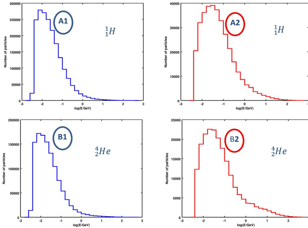
**Figure 1.** The spectra of  $\log(E/\text{GeV})$  of the EAS particles generated by CORSIKA 7.6900 for each of the light atomic mass extraterrestrial nuclei selected for this study. The left column are the whole spectra, and the right column are the no-photons spectra.
