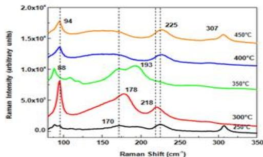
**Fig. 2:** Raman spectra of SnS thin films deposited at different substrate temperatures.
