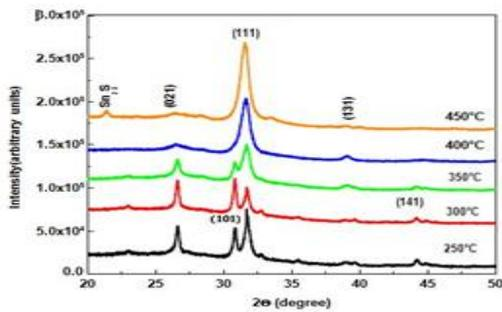
**Fig. 1a:** X-ray diffraction spectra of SnS films deposited at different substrate temperatures.
