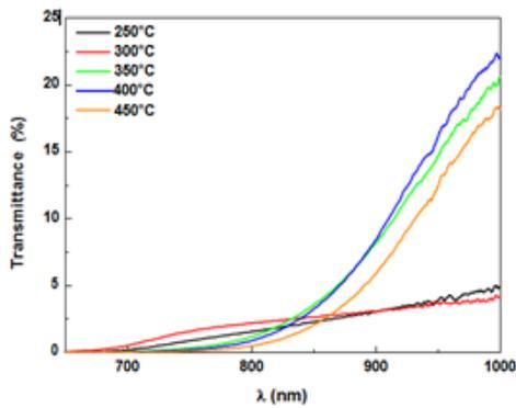
**Fig. 5:** Optical transmission spectra of SnS thin films deposited with different substrate temperatures
