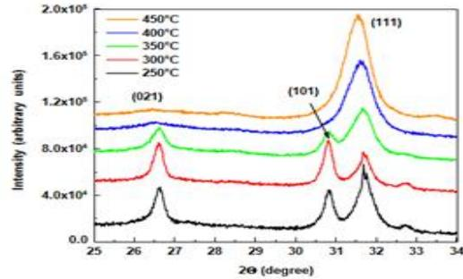
**Fig. 1b:** Detail of the X-ray diffraction spectra of SnS thin films clearly showing the (111) peak.
