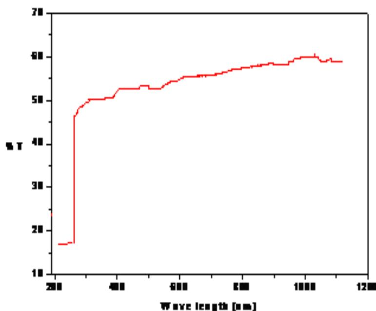
Fig.3: UV-visible transmittance spectrum for gamma-glycine crystal
