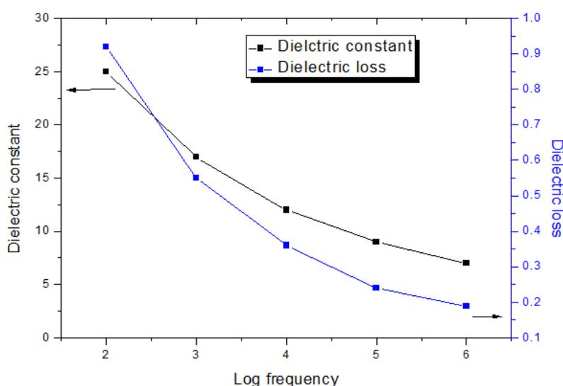
**Fig.2:** Variations of dielectric constant and dielectric loss as a function of frequency for the grown gamma-glycine crystal
