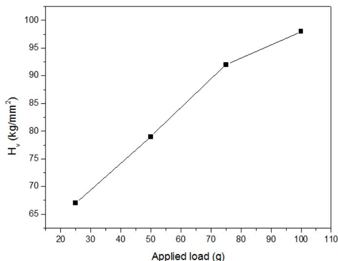
**Fig.1:** Variation of hardness number with the applied load for gamma-glycine crystal
