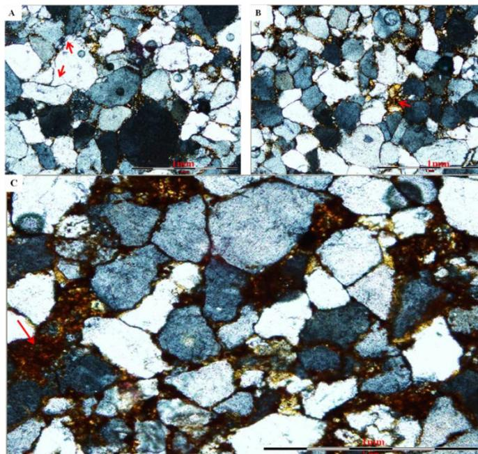
**Figure 16:** Photomicrographs for Mn-Fe coated terrigenous clasts with red arrows to indicate. a) Diagenetic quartz overgrowth. b) Calcite cements reflecting high bright yellow interference colour under cross polarized light. The whole bar represents 1mm for a scale.
