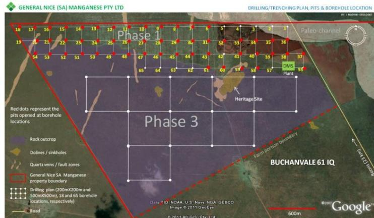
Figure 8: Exploration plan map showing open pits and borehole location in the mine area.
