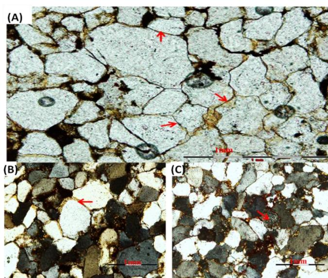
**Figure 15:** SEM-EDX image and photomicrographs of the Mn-Fe coated terrigenous clasts, arrows for indications. a) Weak to absence of hematite coating at grain contact as an indication of diagenetic origin for iron oxide. b) Clearly discernible iron oxide coating forming a ring round detrital quartz grain. c) A bright speck indicating alteration of feldspar grain.
