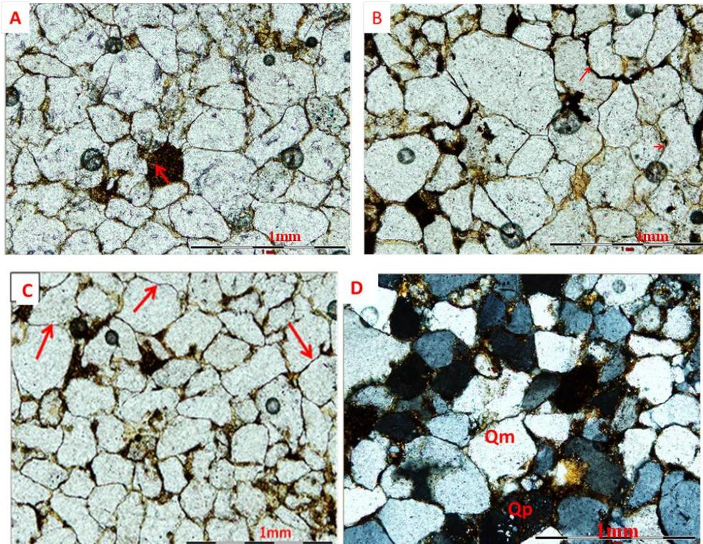
Figure 9: Photomicrographs for Mn-Fe coated terrigenous clasts in mining area, arrows for indications. a) Volcanic lithic fragment. b) Concave-convex contacts between neighboring framework grains. c) Long and embayed contacts between framework grains indicating a moderate degree of compaction and d) Monocrystalline (Qm) and polycrystalline (Qp) quartz grain captured under cross polarized light.
