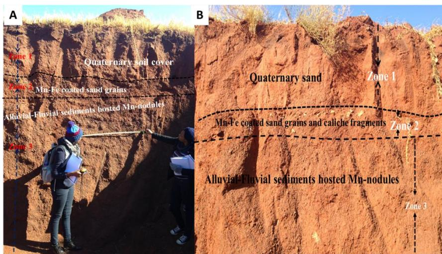
**Figure 5:** Soil profile setting in the mine area subdivided into three varieties of zones (Zone 1, Zone 2 and Zone 3) on the basis of difference in mineral composition and macroscopic constituents.
