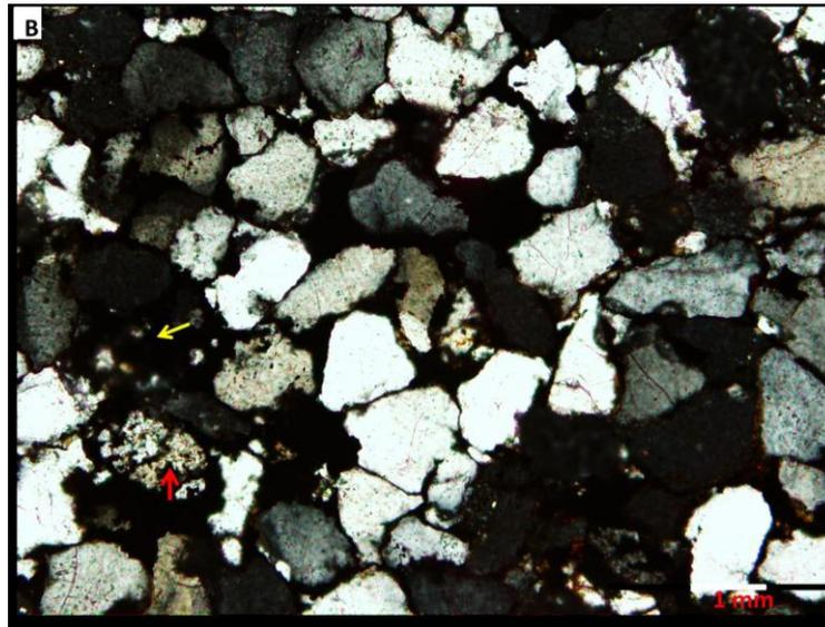
**Figure 18:** Photomicrograph shows Mn-oxide coated clast and also shows framework grains floating in the Mn-oxide cement. Red arrow indicates chert partially replaced by Mn oxide, and the yellow arrow indicates a grain was nearly completely replaced by Mn-oxide, remaining only little part.
