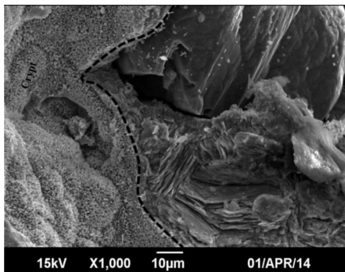
**Figure 17:** SEM photomicrograph of manganese bearing nodule indicating the pseudomorphic texture of cryptomelane in cavities after replacement of clay minerals.
