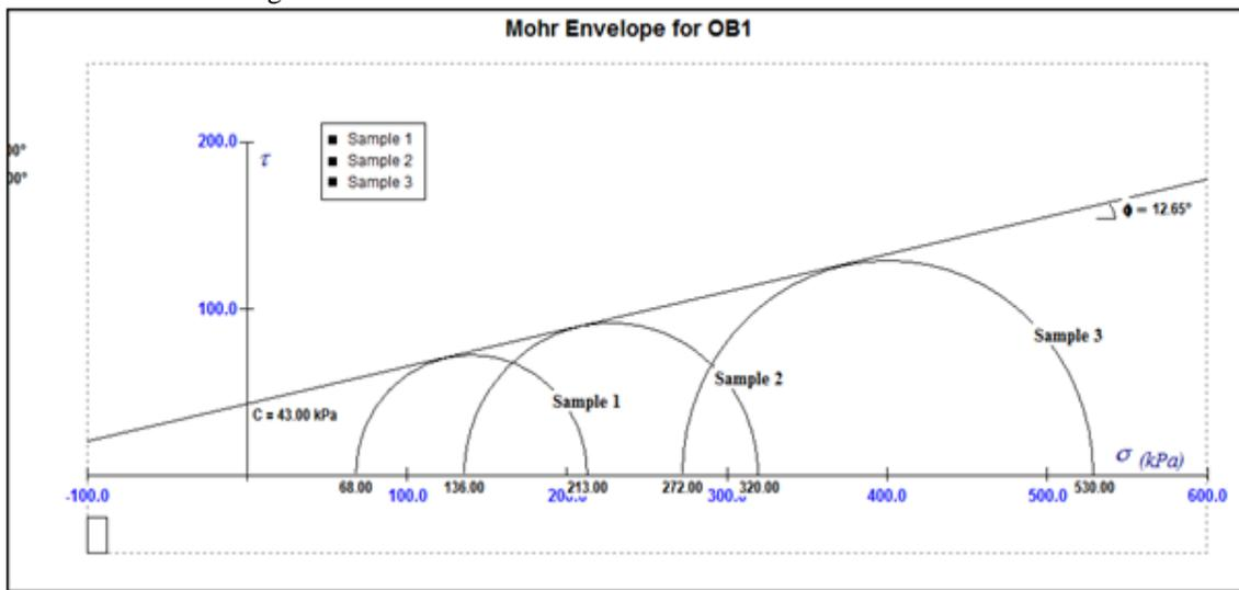
**Fig. 11 Triaxial test plot showing the mohr envelope, cohesion and friction angle.**
