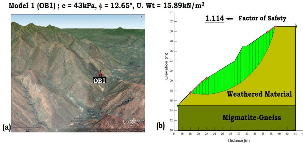
**Fig. 13 Geostudio Model diagram of the slide at OB1.**
