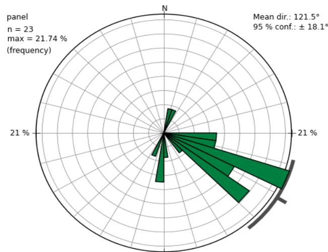
**Fig. 4 Rose diagram showing the orientation of joints in the area.**
