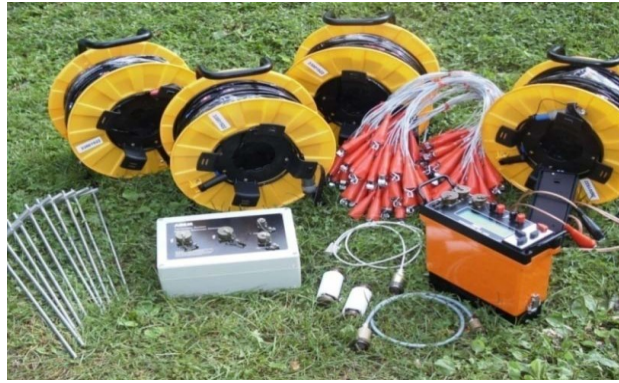
Fig. 2: SAS 1000/4000 Terrameter unit used for electrical resistivity survey (ERS) consisting of electrodes, electrode cables and control unit
