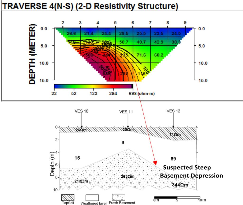
Figure 6: 2-D resistivity structure and geo-electric section for Traverse 4
