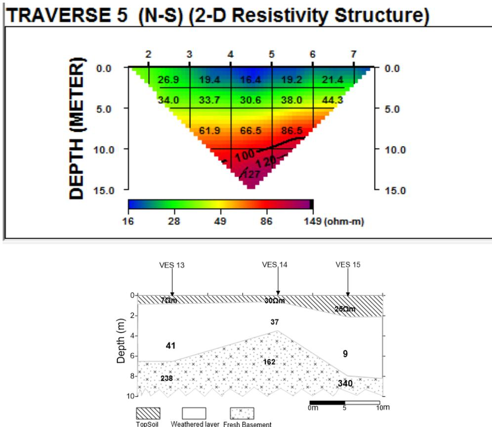
Figure 7: 2-D resistivity structure and geo-electric section for Traverse 5
