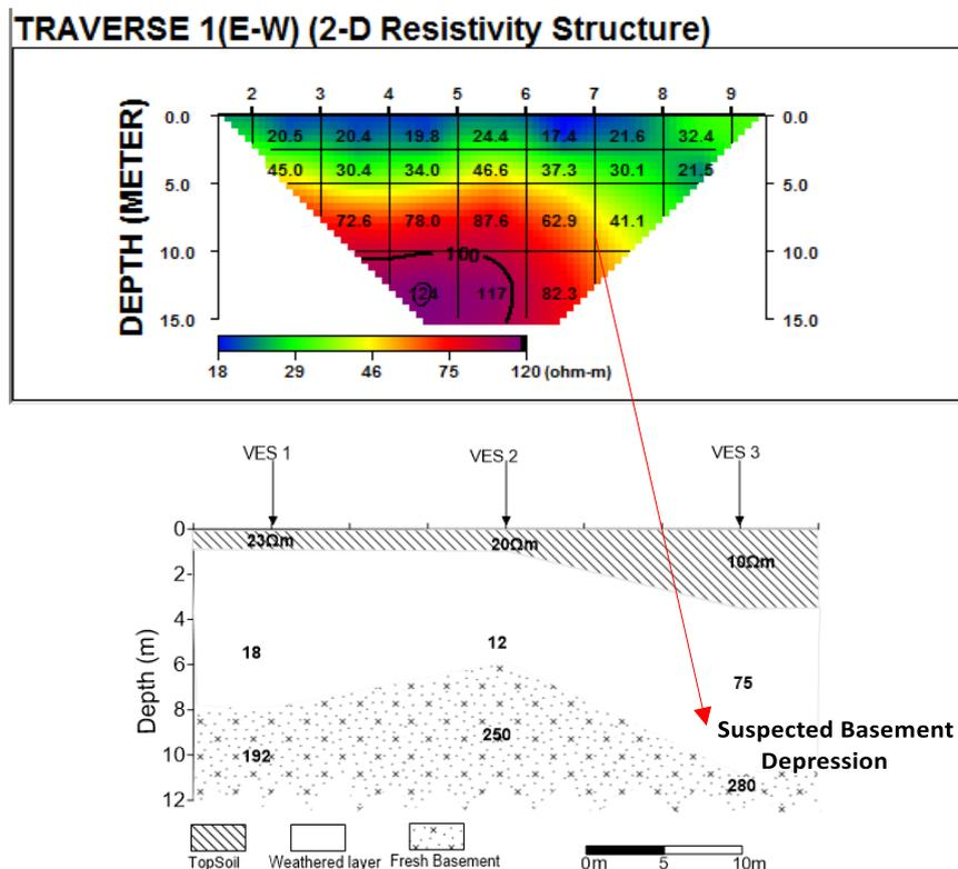
**Figure 3: 2-D resistivity structure and geo-electric section for Traverse 1**
