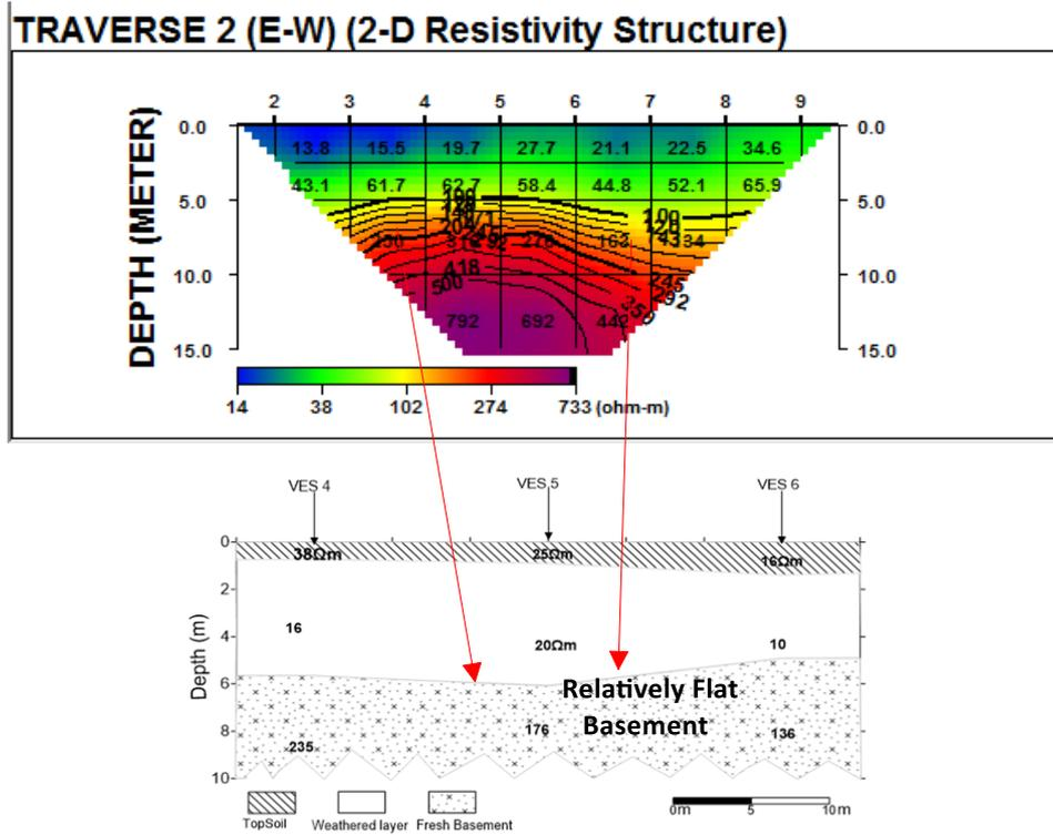
Figure 4: 2-D resistivity structure and geo-electric section for Traverse 2
