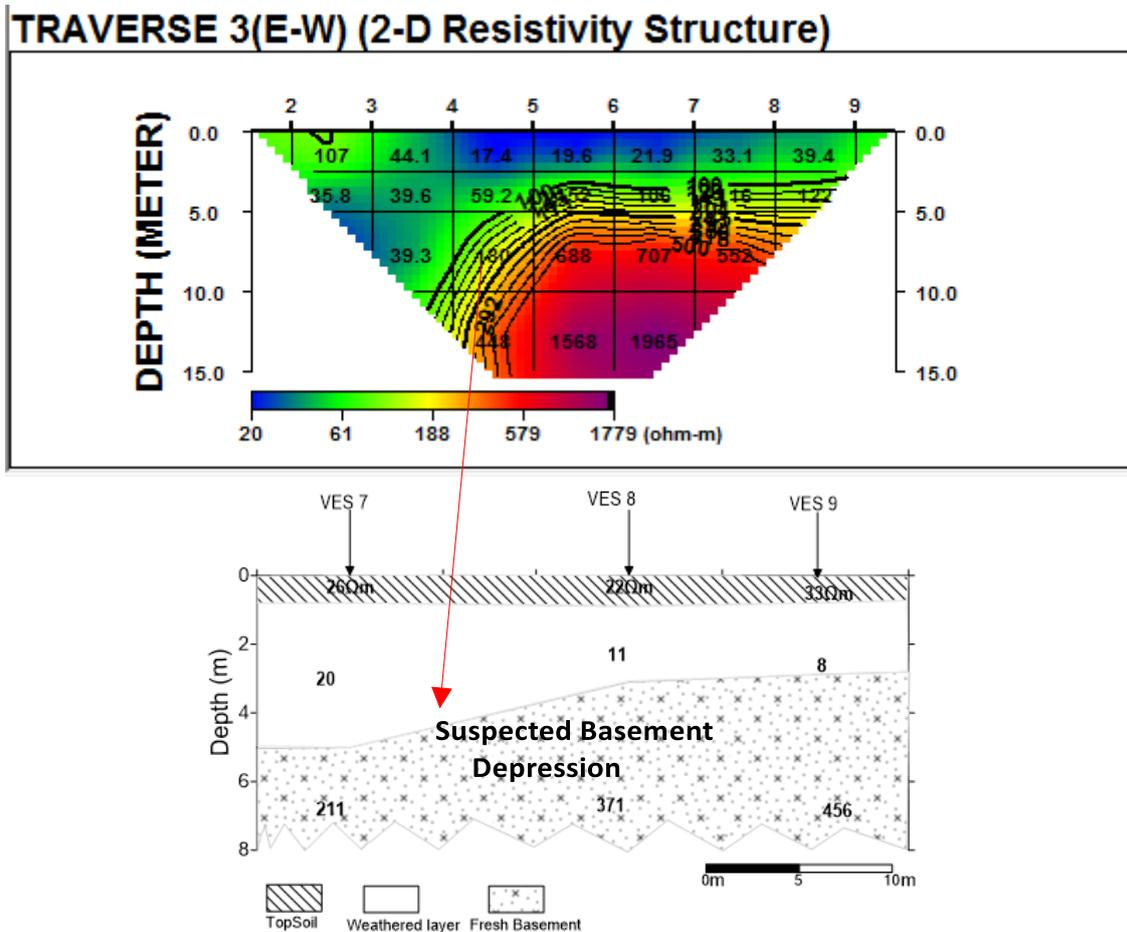
Figure 5: 2-D resistivity structure and geo-electric section for Traverse 3
