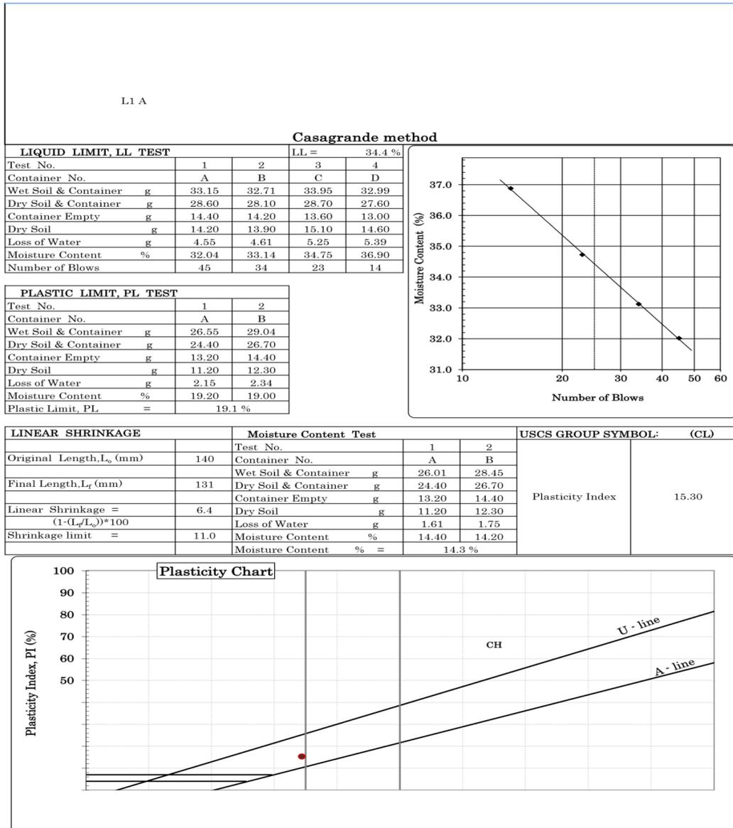
Figure 10: Atteberg limits chart (Liquid limit, Plastic limit and Plasticity index) for location 1
