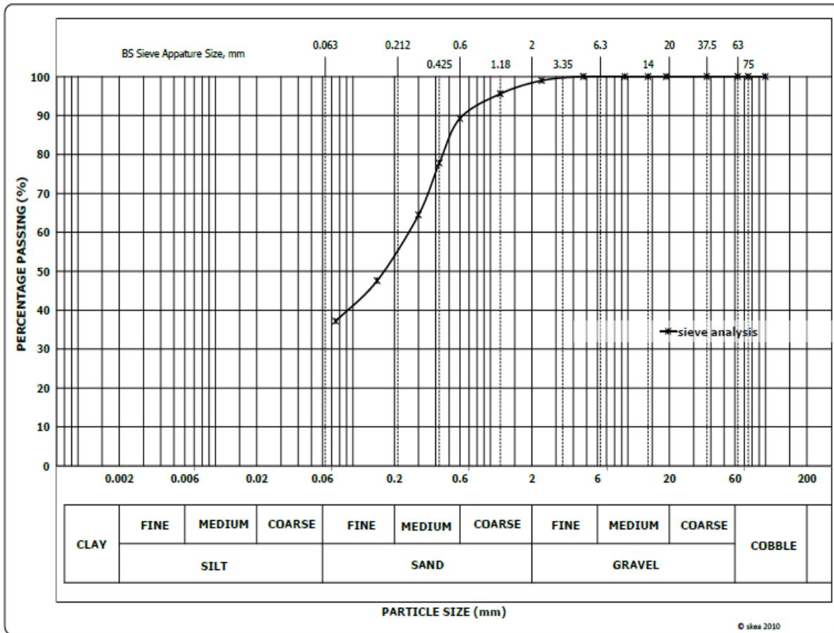
Figure 9: Particle size distribution graph for location 2
