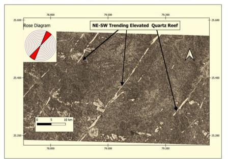
Figure 5. The Quartz Reef in the Bundelkhand Granitic Massif is shown in Block II, represented by lightcolored NE-SW lines in the DEM.
