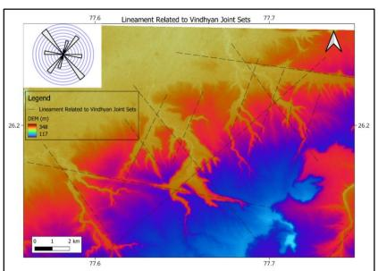
Figure 4. In Block I, depicting the Vindhyan Rock Exposures, The DEM also displays lines of depressed areas, which are marked by dashed lineaments.
