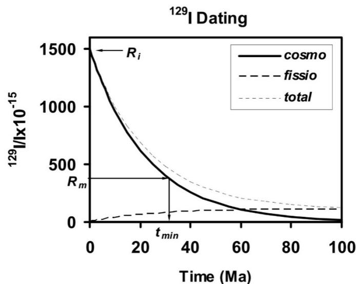
**Fig. 15.** Iodine dating: Systematics of the decrease of cosmogenic and build-up of fissiogenic  $^{129}\text{I}/\text{I}$  ratios. The cosmogenic (marine)  $^{129}\text{I}/\text{I}$  ratio decays from the input ratio  $R_i = 1500 \times 10^{-15}$ . Arrows indicate the determination of  $t_{\min}$  from the measured ratio  $R_m$  using the decay curve of cosmogenic  $^{129}\text{I}/\text{I}$  (Fehn et al., 2007).
