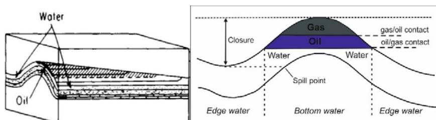
**Fig. 1.** Relationship between oil, gas and water in an anticline trap
