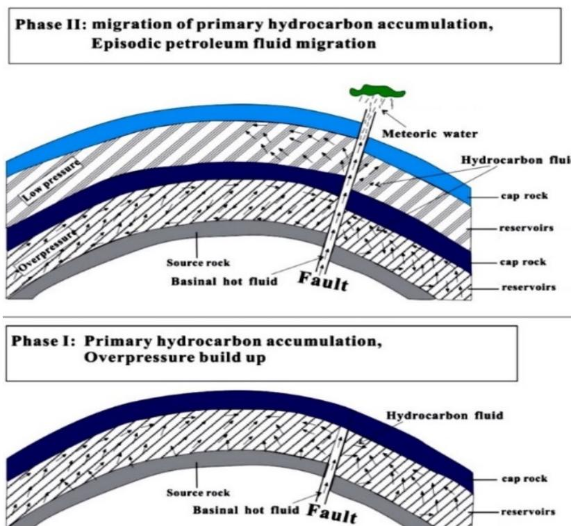
Fig. 4. Schematic model for episodic fluid migration in the fault-zone area (Jin et al., 2008)
