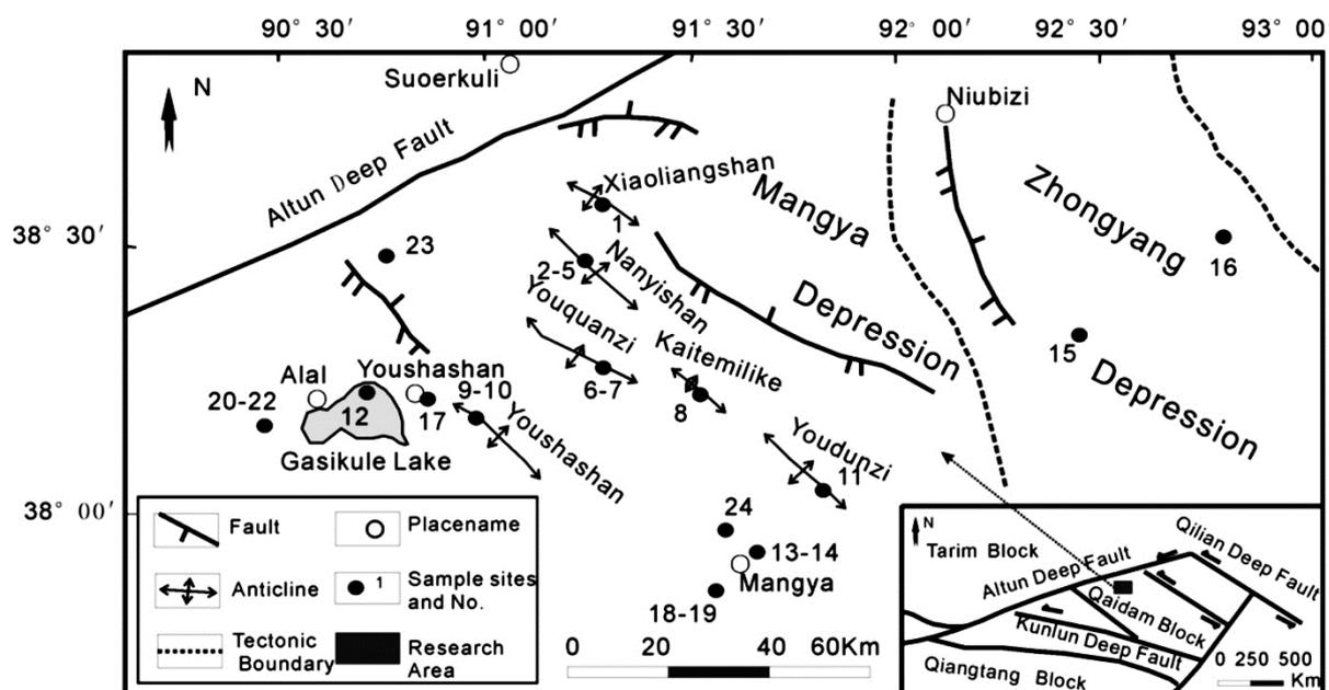
Fig 17. Location of the western Qaidam basin and distribution of its main anticlines, oilfield bins and sample sites (Tan et al., 2011).
