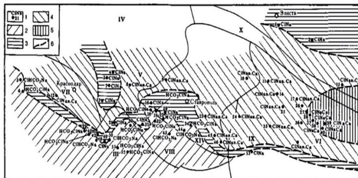
**Fig. 2.** A hydrogeochemical map: 1. No. of water point and chemical composition formula by the component precedence; zones of water distribution with composition: 2.  $\text{HCO}_3\text{-Cl-Na, Cl-HCO}_3\text{. Na}$ ; 3.  $\text{Cl-Na}$ ; 4.  $\text{Cl-Na-Ca}$ ; 5.  $\text{Cl-Na-Ca}$ ; 6. Zone boundary (Tikhomirov, 2016)
