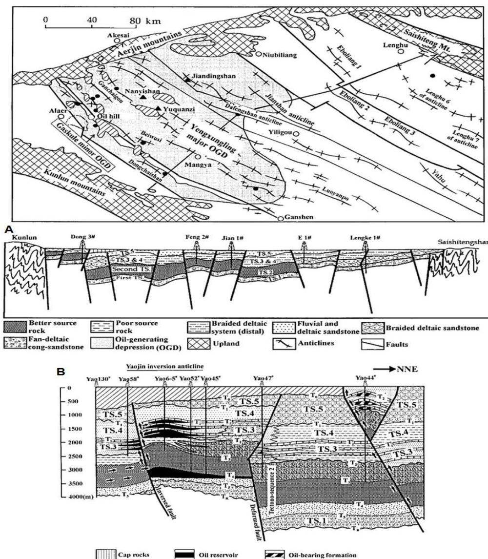
**Fig. 22.** A: Distribution map of oil-generating depression and anticline in western Qaidam basin, B: (B) Yaojin-Youshashan (oil hill) cross section, showing the reversed structures formed by basin tectonic inversion processes (from Xia et al., 2001)
