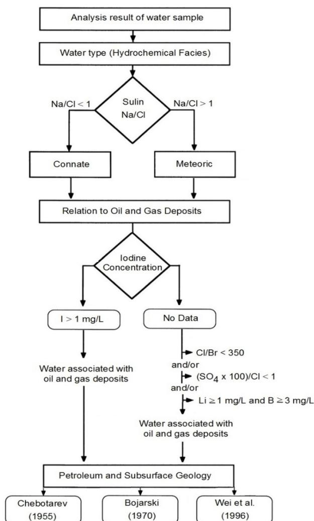
Fig. 23. Systematic work flow chart proposed for high-accuracy estimation with hydrochemical methods of oil and gas deposits in a wildcat sedimentary basin
