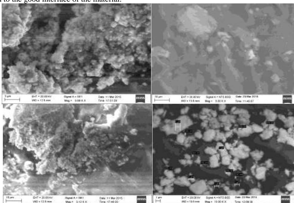
**SEM Images of OMMT Castor- based epoxy nanocomposites**
