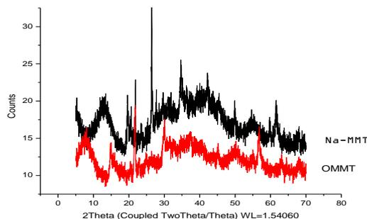
XRD Spectrum Of Na-MMT and OMMT
