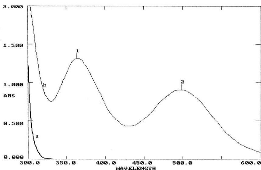
Fig .4 Absorption spectrum of reaction product of Isoxsuprine and iodine
