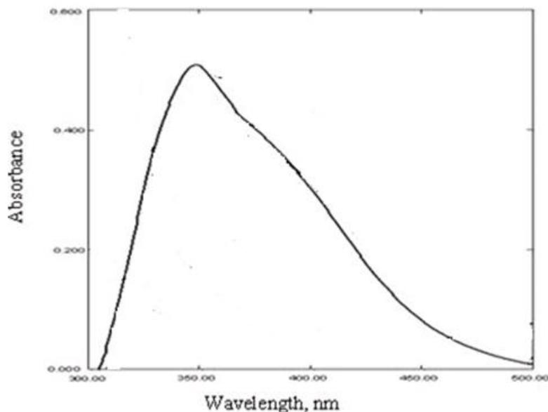
Fig .3 Absorption spectrum of reaction product of Isoxsuprine and p-CA
