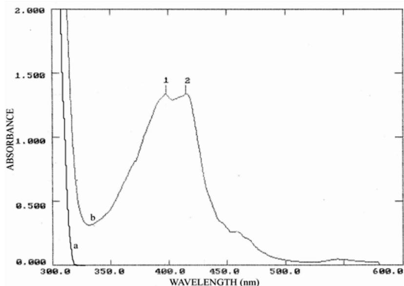
**Fig .2** Absorption spectrum of reaction product of Isoxsuprine and TCNE
