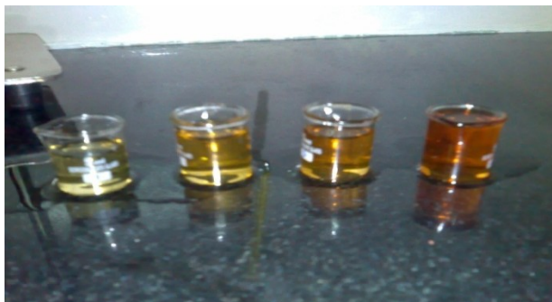
Colloidal suspension of CdSe quantum dots of increasing size
