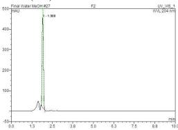
HPLC: Experimental Parameters: Column: Acclaim<sup>TM</sup> C-18, 5 $\mu$ , 4.6 × 250mm, Wavelength: 204nm, Mobile phase: 100% Acetonitrile, Flow rate: 1.5ml/min, Column temperature: 28°C, Injection volume: 20 $\mu$ L, Run time: 10mins, Retention time: 1.9min
