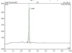
HPLC: Experimental Parameters: Column: Acclaim<sup>TM</sup> C-18, 5 $\mu$ , 4.6 × 250mm, Wavelength: 210nm, Mobile phase: Methanol: Water (85:15 v/v), Flow rate: 1ml/min, Column temperature: 28°C, Injection volume: 20 $\mu$ L, Run time: 10mins, Retention time: 3.6mins
