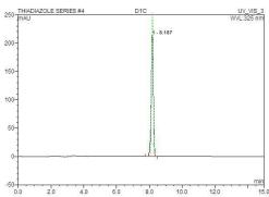
HPLC: Experimental Parameters: Column: Acclaim<sup>TM</sup> C-18, 5 $\mu$ , 4.6 × 250mm, Wavelength: 325nm, Mobile phase: Water: Acetonitrile (60:40 v/v), Flow rate: 1ml/min, Column temperature: 28°C, Injection volume: 20 $\mu$ L, Run time: 15mins, Retention time: 8.1mins
