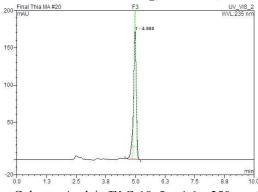
HPLC: Experimental Parameters: Column: Acclaim<sup>TM</sup> C-18, 5 $\mu$ , 4.6 × 250mm, Wavelength: 235nm, Mobile phase: Methanol: Water (80:20 v/v), Flow rate: 1ml/min, Column temperature: 28°C, Injection volume: 20 $\mu$ L, Run time: 10mins, Retention time: 4.9min
