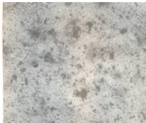
Figure 8. Effect of thermoxidative aging on AR control coating (a) before and (b) after aging at 100°C
