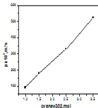
Fig.6 Influence of feed concentration on permeability coefficient per 100 ml of Pb(II). P: 0.1M NaNO<sub>3</sub>, 0.02M Pb(II), M: cyanex302/xylene, 0.02M DPTA, 1M NaCl.
