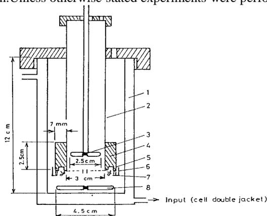
**Fig.1. Scheme of Pertraction apparatus: (1) double shield glass outer vessel, (2) Plexiglas inner tube, (3) Teflon cross stirring blade, (4) Teflon holder, (5) silicon rubber ring, (6) niobium holder, (7) titanium holder, (8) magnet**
