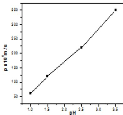
Fig.3 Influence of feed acidity on permeability coefficient per 100 ml of Pb(II). P: 0.1M NaNO<sub>3</sub>, 0.02M Pb(II), M: 0.1 g/ml cyanex302/xylene, 0.02M DPTA, 1M NaCl.
