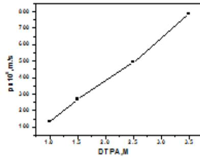
Fig. 2 Influence of carrier concentration on permeability coefficient  $p \times 10^5$  in  $m/s$  of  $Pb(II)$ .  $P: 0.1M$ ,  $NaNO_2: 0.02M$ ,  $Pb(II): 0.02M$ ,  $cyanoex302/xylylene: 0.02M$ ,  $DTPA: 0.1M$ ,  $NaCl$ .
