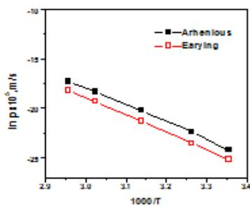
Fig. 2 Influence of temperature on permeability coefficient  $\ln p \times 10^5$  in  $m/s$  of  $Pb(II)$ .  $P: 0.1M$ ,  $NaCl: 0.02M$ ,  $Pb(II): 0.02M$ ,  $cyanoex302/xylylene: 0.02M$ ,  $DTPA: 0.1M$ ,  $NaNO_3$ .
