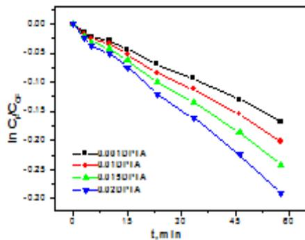
Fig. 2.8 In-lagerithmic plot of  $\ln(C_i/C_0)$  against time, in different DTPA concentrations.  $P: 0.1M$ ,  $NaNO_2: 0.02M$ ,  $Pb(II): 0.02M$ ,  $cyanoex302/xylylene: 0.02M$ ,  $DTPA: 0.1M$ ,  $NaNO_3$ .
