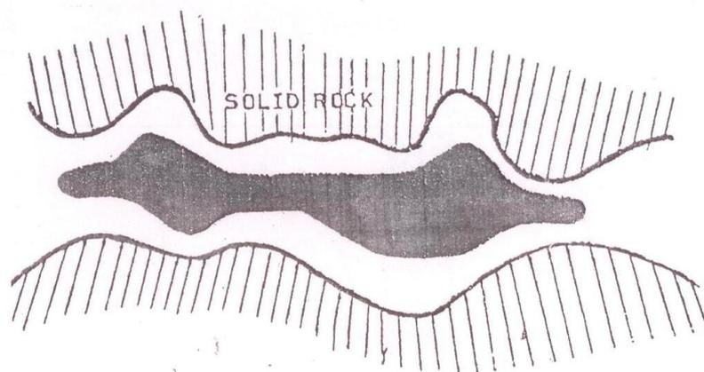
**Figure-1** The effect of interfacial tension on the movement of oil ganglia through narrow neck of Rock Pores.
