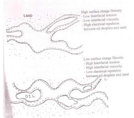
Figure-6 The effect of surface charge density of oil/brine interface on the oil displacement process
