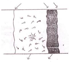
Figure-2 Displaced oil ganglia must coalesce to form a continuous oil bank
