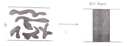
Figure-3 An efficient propagation of an oil bank through Porous media
