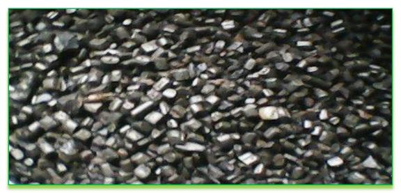
Plate II: Granular Activated Carbon after remediation
