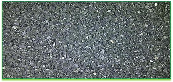
Plate I: Granular Activated carbon before remediation
