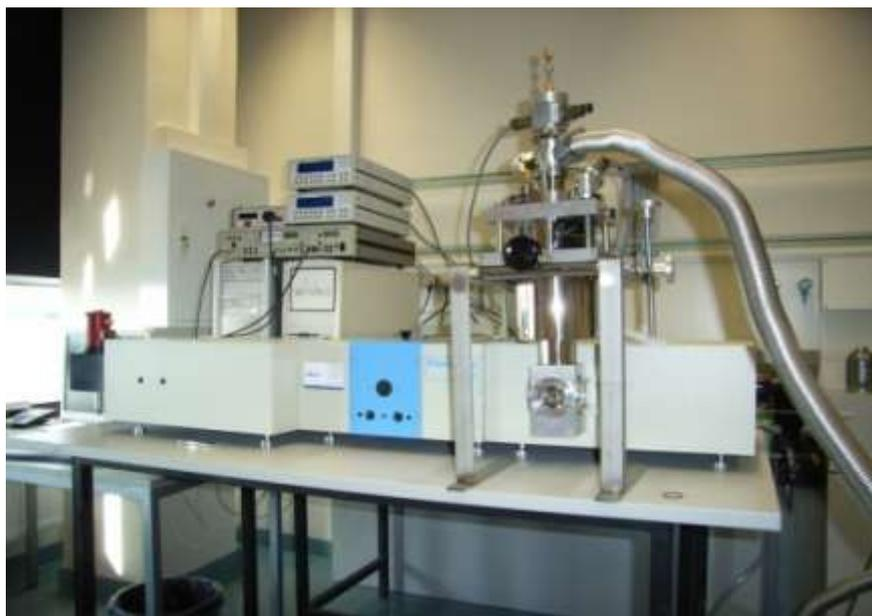
figure 2: Fluorolig-3 (FL3-22) Spectrofluorometer
