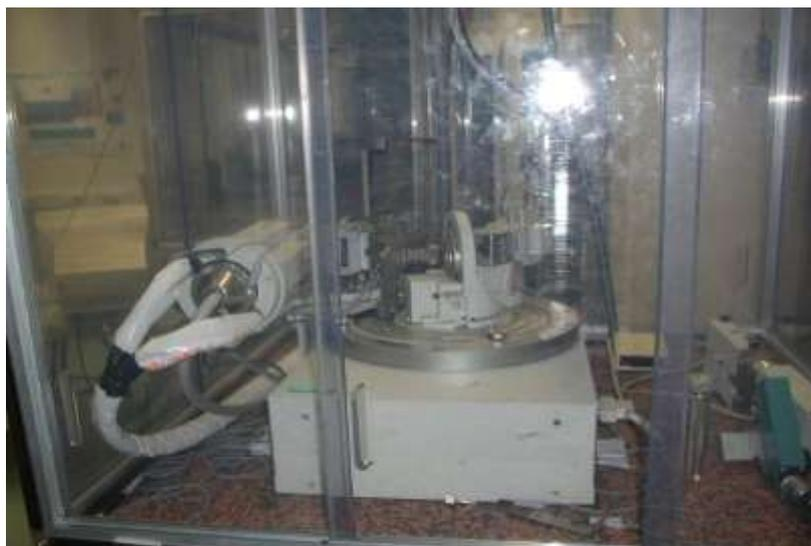
figure 1: X-Ray Powder Diffractometer (D5000)
