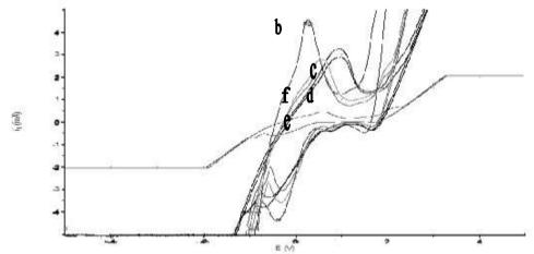
Figure 2. Cyclic voltamograms of (a) stainless steel and (b-f) Fe1-5-Co-Ni/s electrodes on water electrolysis by adding 5 g of NaHCO<sub>3</sub> in one liter water
