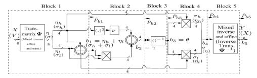
Fig. 1. The S-box (the inverse S-box) using composite fields and polynomial basis and their fault detection blocks.
