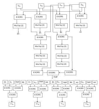
Fig. 4. Inverse mix columns operation
