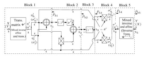
Fig. 2. The S-box (the inverse S-box) using composite fields and normal basis and their fault detection blocks.
