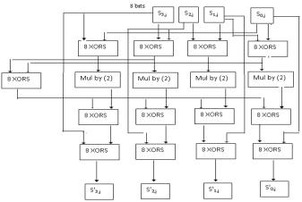
Fig. 3. Forward mix columns operation
